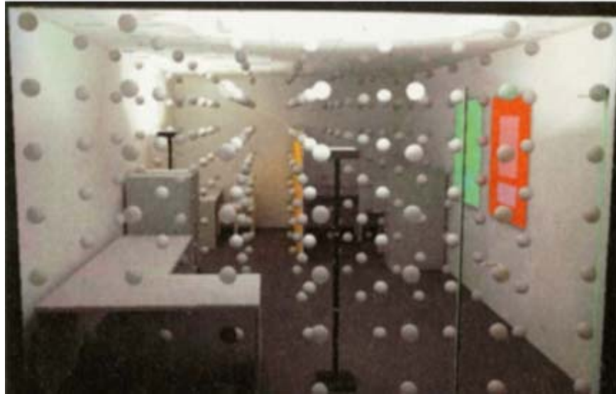
FIGURE 3 IRRADIANCE VOLUME THE SPHERES REPRESENT THE AMOUNT OF LIGHT AT A POINT [IMAGE FROM GREGER98]
